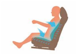
Newly adopted front-seat ventilation system draws hot and humid air away from areas where the occupant's body is in contact with the seat surface, providing a more comfortable driving environment. The system offers three-stage control over ventilation strength.
