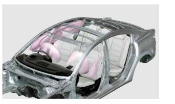
A full complement of airbags – front, front seat side, curtain – provide another layer of protection in depth against physical shock and injury in a collision.
