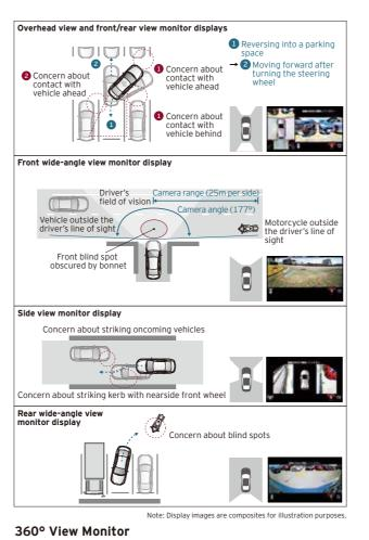
Four cameras on the front, sides and rear of the vehicle show the area around the car on a central display. Combined with alarm sounds triggered by eight parking sensors at the front and rear, the system helps you to avoid danger when pulling into or out of a garage, approaching T-shaped intersections or passing an oncoming car on a narrow road.
