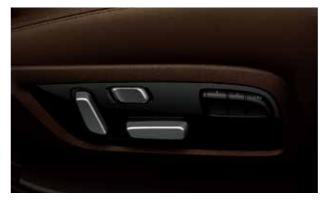
Ten-way power driver's seat with fore/aft slide, recline, lumbar support, lift and tilt provides the optimum driving position for drivers of almost any size. The memory saves multiple seating positions along with the projection location, brightness and content setting of the Active Driving Display.
