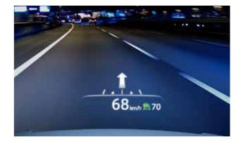
The windscreen-type Active Driving Display is divided into two zones for better legibility with high-priority vehicle-status information and advanced safety information shown in the lower section, and driving environment information such as turn-by-turn directions in the upper section.
