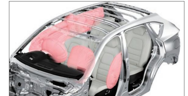
A full complement of airbags – front, front seat side, curtain – provide another layer of protection in depth against physical shock and injury in a collision.
