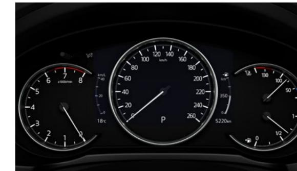
The three-meter cluster features a seven-inch TFT LCD colour display in the centre. In addition to vehicle speed, it shows diversified vehicle information in a clear, easy-to-read manner near the centre of the driver's line of sight.
