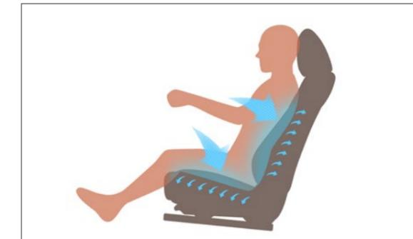
Newly adopted front-seat ventilation system draws hot and humid air away from areas where the occupant's body is in contact with the seat surface, providing a more comfortable driving environment. The system offers three-stage control over ventilation strength.
