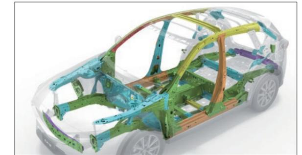
The body provides excellent collision safety performance. Extensive use of ultra-high-tensile steel gives strength with low weight, while the framework absorbs and channels energy away from the cabin.
